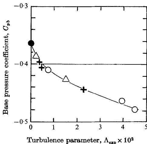
FIGURE 4. Base pressure coefficient as a function of free-stream turbulence parameter.  $\circ$ ,  $D = 5$  cm;  $+$ ,  $D = 10$  cm;  $\Delta$ ,  $D = 15$  cm;  $\bullet$ , all values of  $D$ .
