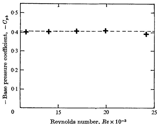
FIGURE 3. Base pressure coefficient as a function of Reynolds number for a fixed value of the free-stream turbulence parameter ( $\Lambda_{\text{exp}} = 0.049$ ) and  $D = 10$  cm.
