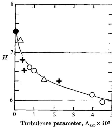
FIGURE 2.  $H$  as a function of free-stream turbulence parameter.  $\circ$ ,  $D = 5$  cm;  $+$ ,  $D = 10$  cm;  $\triangle$ ,  $D = 15$  cm;  $\bullet$ , all values of  $D$ .
