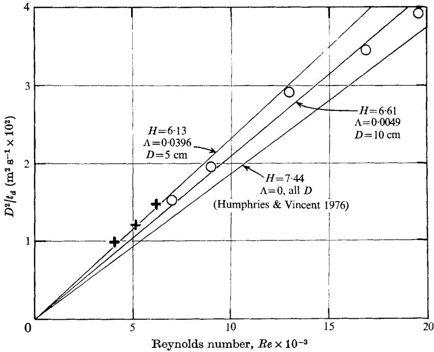
FIGURE 1. Experimental plot of  $D^2/t_d$  as a function of Reynolds number for various values of free-stream turbulence parameter.
