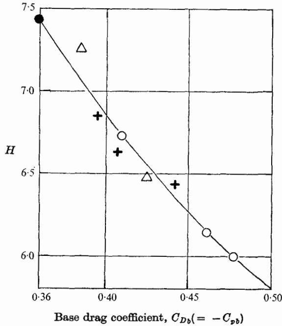
FIGURE 8. Graph to show the relationship between  $H$  and base drag coefficient.  $\circ$ ,  $D = 5$  cm;  $+$ ,  $D = 10$  cm;  $\triangle$ ,  $D = 15$  cm;  $\bullet$ , all values of  $D$ . —,  $H = 9.15/(C_{Db} + 0.76)^2$ .
