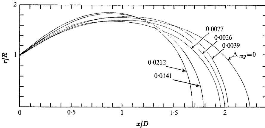
FIGURE 5. Experimentally determined wake-bubble boundaries for various values of free-stream turbulence parameter.
