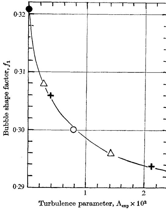
FIGURE 7. Bubble shape factor as a function of free-stream turbulence parameter.
