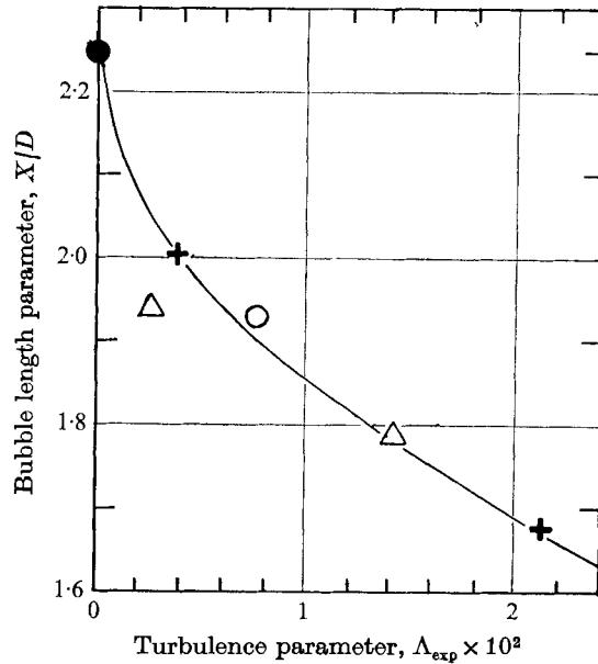
FIGURE 6. Bubble length parameter as a function of free-stream turbulence parameter.  $\circ$ ,  $D = 5$  cm; +,  $D = 10$  cm;  $\triangle$ ,  $D = 15$  cm;  $\bullet$ , all values of  $D$ .
